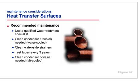
Optimum performance of heat transfer components depends on keeping the heat transfer surfaces free from scale and sludge. Even a very thin deposit of scale can substantially reduce heat transfer capacity. Owners of water-cooled chillers should engage the services of a qualified water treatment specialist to
